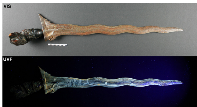
Figure 2. Keris (Ilc 2118) from the MKB under visible light (VIS) and under ultraviolet fluorescence (UVF) revealing the synthetic oil coating (FTIR analyzed). © JM, HE-Arc/MKB 2020
