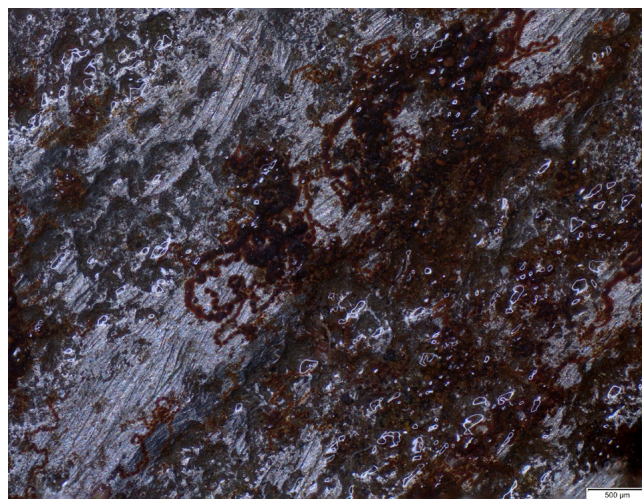
Figure 10. Filiform corrosion under acrylic coating (FTIR analyzed) on keris blade (Ilc 22217) from the MKB (20× magnification).
