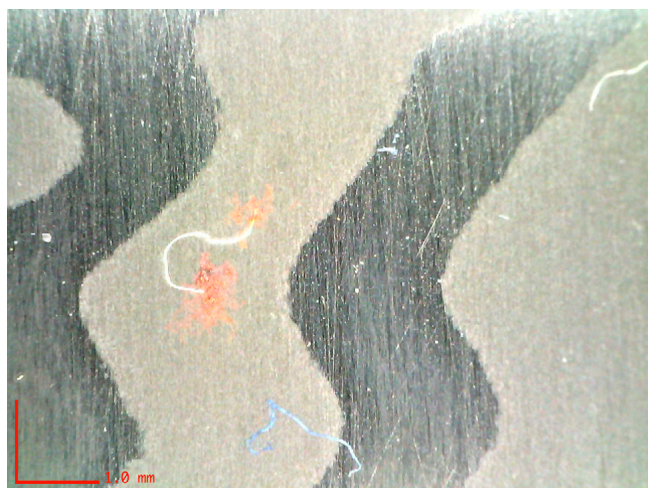
Figure 9. Dust particle on pamor coupon with paraffin oil coating (4) and localized corrosion development (50× magnification)
